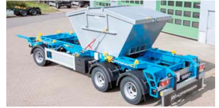
One container at the load centre of gravity.
